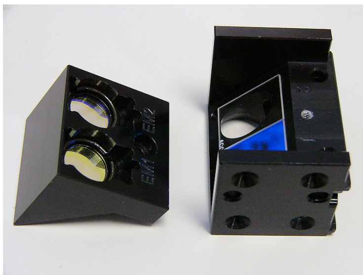
Figure 4-6: Filter cube with the top removed (left), exposing the mirrors (right)
